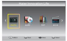
Please make sure that the USB device have plugged in the slot. There are four type media item can be selected, such as photo, music, Movie and text. Select the type media item by pressing  $\P \triangleright$ , press **OK** button to enter the disk selection menu.
